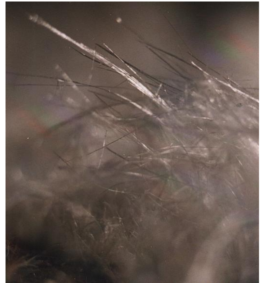
Microscopic, needle-like crystals fill the naturally occurring pores and capillary tracts of concrete for guaranteed waterproof structures.
